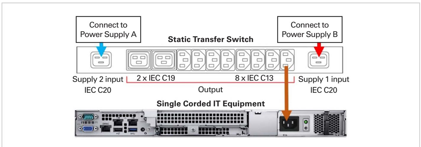
STS units can be requested via ONEDC. If providing your own STS, written permission from NEXTDC is required to ensure the unit has overlapping switching of the neutral conductor.
